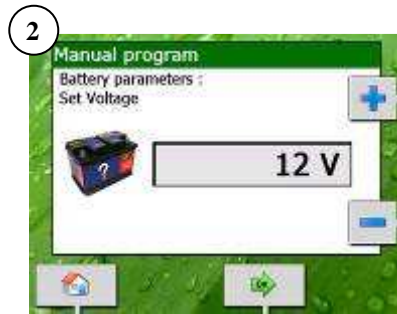
Set battery voltage
